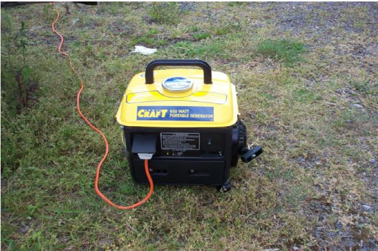
A typical two stroke petrol generator. Gives 230V / 12V at 650 W.
