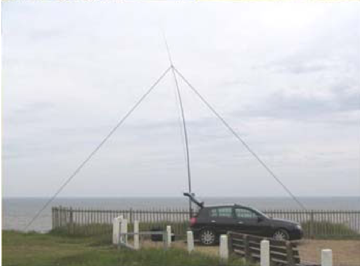
Top left: Typical operating position Top right: 40M inverted V Bottom: Another view of 40M inverted V
