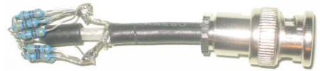
The M6RHB dummy load. Resistors purchased from an East German bread shop.
