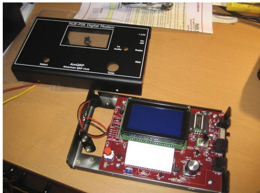
Power came up again and stayed on this time. I was looking for the boot-sequence on the display. Nothing! Just nothing. The screen was on, but no cursor or boot message. Perhaps the crystal is not oscillating and without a 10MHz clock agitating the microprocessor it most likely doesn't feel compelled to move beyond instruction #1. So I touched across the two pins of the crystal, hoping to change the parallel capacitance enough to get it going. Nothing!
